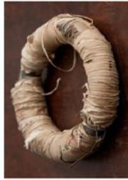
While Faraday describes the making of the ring in its entirety here, the actual work would probably have taken much longer. A modern experiment to build a replica induction ring using original materials took 10 working days.
