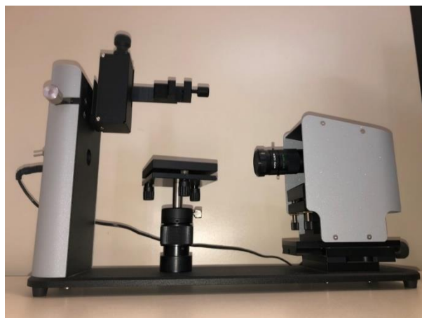
Figura 6 – Tensiômetro óptico (One Attention – Theta Instrument)
