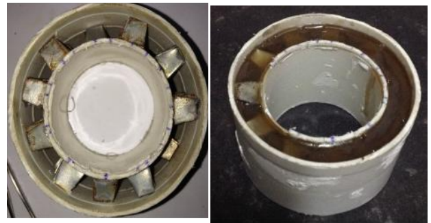
Fig. 7. Modulators. (a) Mold. (b) Mold with Epoxy resin.
