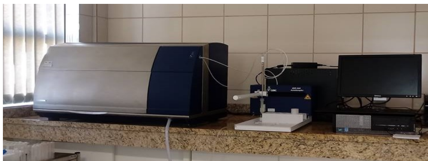
Figura 17- WineScan™ SO 2 (FOSS ® , Dinamarca)
