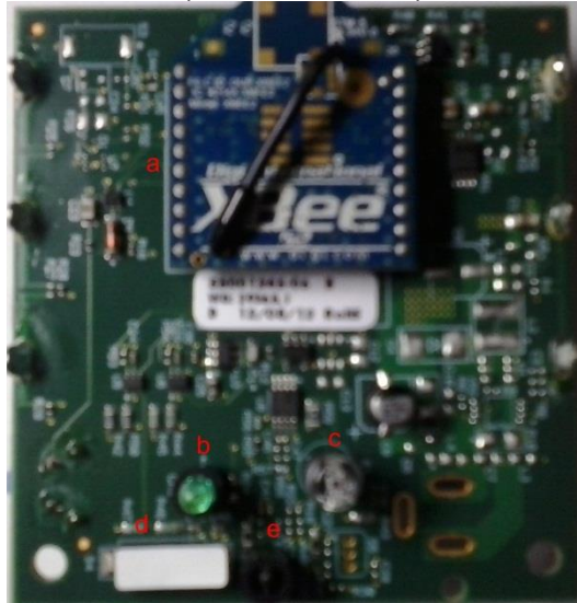
Figura 43 - Sensor XBee ZB L/T/H (XS-Z16-CB2R)
