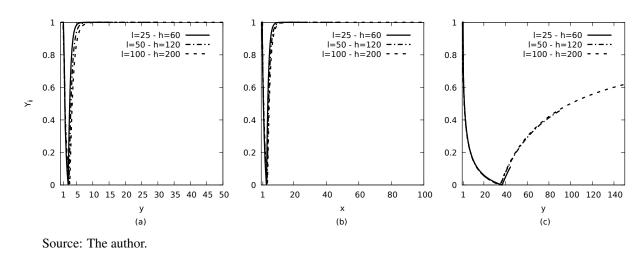
Figure 15 – Dependence of domain size: Mass Fraction for (a) inflow, (b) center and (c) outflow axes.
