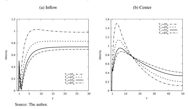
Figure 30 – Dimensionless absolute velocity distribution.
