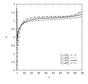
Figure 33 – Dimensionless pressure distribution in the outflow axis.
