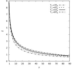
Figure 21 – Mixture fraction distribution in the outflow axis.
