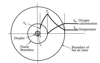
Figure 2 – Schematic diagram of a droplet combustion process.
