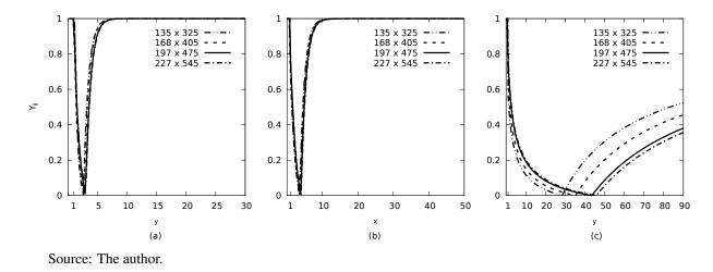
Figure 13 – Test mesh dependence: Mass fraction for (a) inflow, (b) center and (c) outflow axes.
