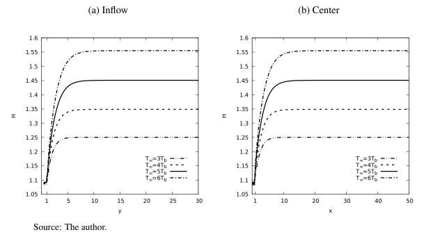
In the distribution showed in Fig. 23, the enthalpy excess keeps increasing until the
