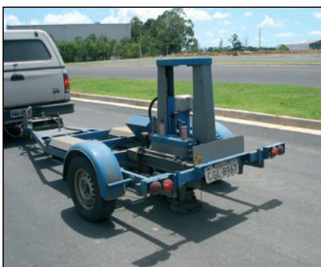
Figura 5 – Vista geral do FWD Dynatest
