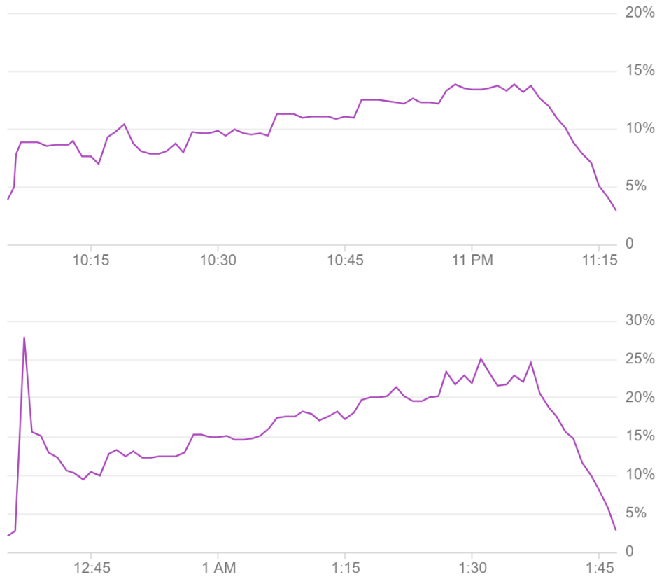
Figure 12 – CPU usage of the Testbed with LoadSun (above) and JMeter (bellow).
