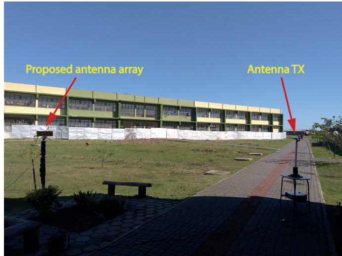
Fig. 38: Picture of the setup. Highlighted on the right it is the Tx antenna and on the left the proposed antenna array.
